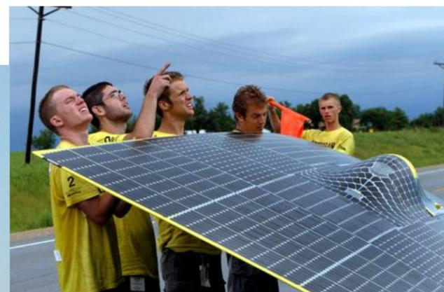
For two hours in the morning and evening, teams are able to charge their batteries using the solar car's array. Many teams have an array stand to angle the solar array toward the sun for maximum exposure. Teams also use these non-raycing
