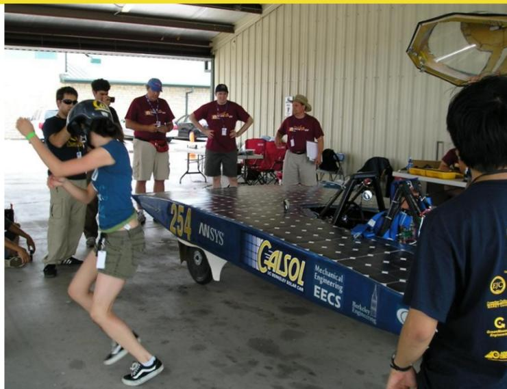
Scrutineering is also about testing the abilities of the drivers. All drivers must pass the egress test, which requires drivers to get out of the car unassisted in 10 seconds or less. Drivers are randomly selected to complete the dynamics tests, which are as much about testing the car's braking, turning, and stability as it is about testing the experience of the drivers.
